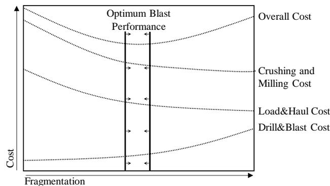
**Figure 2. Mining cost relation (adapted from Efficient Blasting Techniques, (Floyd, 2000))**
